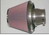
25. Install the silicone hose (084055) onto air filter adapter as shown and secure with the provided hose clamp as shown.
