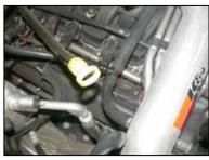
23. Install the provided crankcase vent hose onto the factory crankcase vent fitting and then onto the K&N<sup>®</sup> intake tube as shown.
