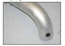
17. Install the provided grommet into the K&N® intake tube as shown.
