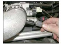
22. Reconnect the air temperature sensor electrical connection as shown.
