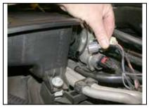
4. Depress the locking tab on the air temperature sensor electrical connection and then pull to disconnect he sensor electrical connection.
