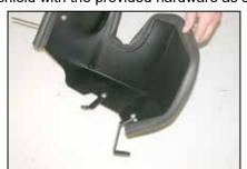
3. Disconnect the stock intake tube from the intake plenum and lift to remove the airbox assembly from the vehicle as shown.
